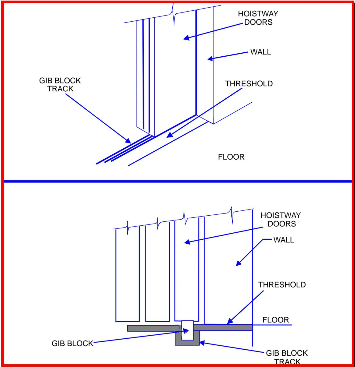
Gib blocks provide stability to the hoistway door as it opens and closes. Normal hoistway doors can be expected to utilize two gib blocks.
